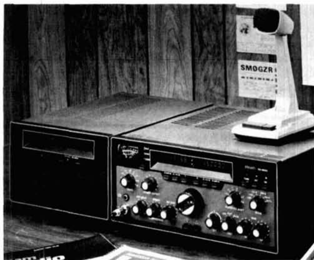
Heath's versatile SS-9000 covers 160 through 10 meters, and can be operated from a computer or smart terminal keyboard just as easily as from its front panel.
